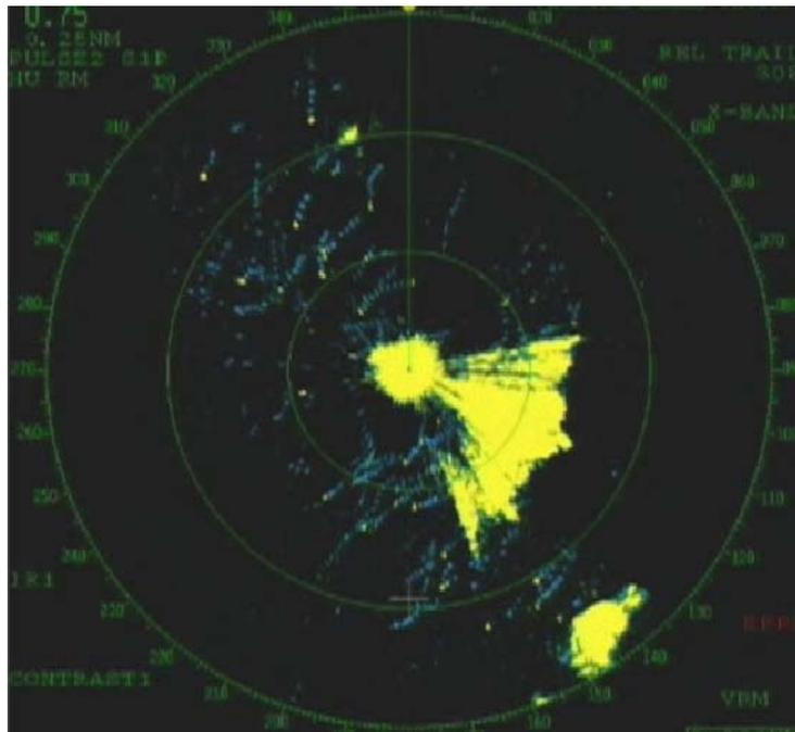
**Figure 3** Example of ground clutter in project area
